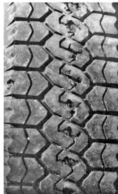
Example of Dyno Damage
